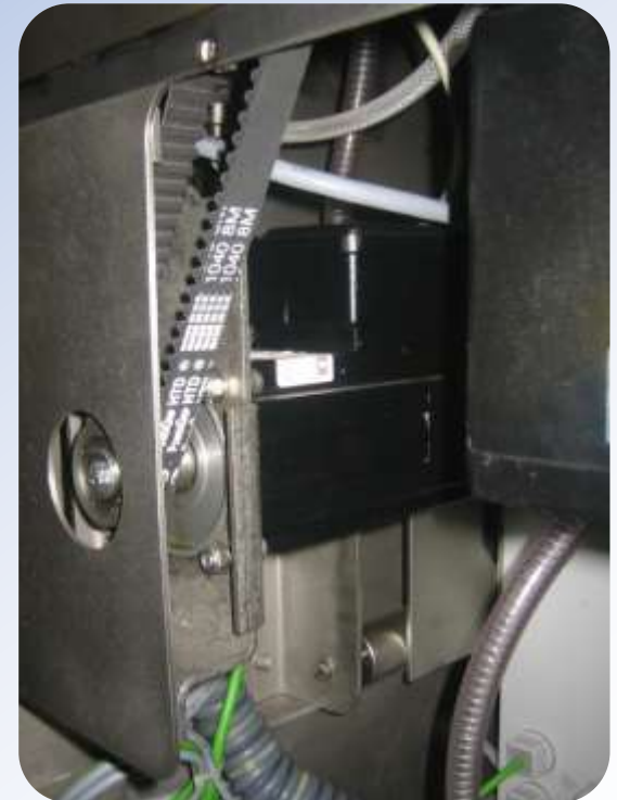
servo twisting drive at „S“ configuration
